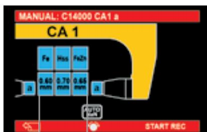
**EN**/ manual setting of up to three materials and up to three thicknesses different from one another
