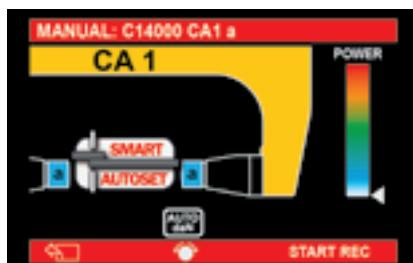
**EN**/ automatic detection of the thickness and the material to be welded
