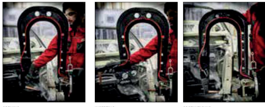
**EN**/ Shark A7 is a revolutionary arm designed to speed up and simplify spot welding operations in the most difficult to access areas. Thanks to the patented "large opening" mechanism, the end section of the Shark A7 opens 90° by simply pressing with your finger, even allowing insertion in boxed or difficult to reach parts.
