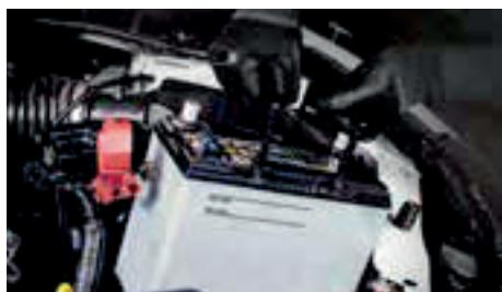
**EN/** Maintenance of the vehicle's electronics power supply during battery changes to prevent loss of settings.
