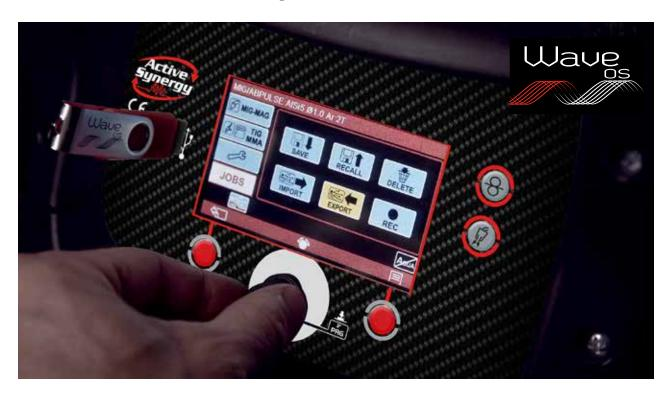
The TFT graphic colour screen is an interface that simplifies product use and makes interaction with the machine immediate. The main parameters (thickness of material to weld and arc correction) are always available to the user for easy display and adjustment.
